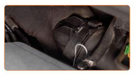
9 Press the air filter cover clips into place.
