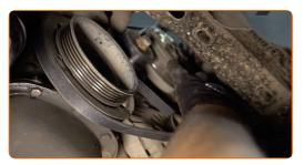
Place the serpentine belt on the crankshaft pulley. Use a drive socket #18. Use a ratchet wrench.
