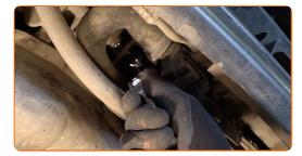
Loosen the upper fastener of the alternator. Use a drive socket #13. Use a drive socket #16. Use a ratchet wrench.
