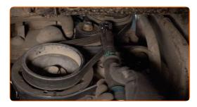
Tighten the upper fastener of the alternator. Use a drive socket #13. Use a torque wrench. Tighten it to 20 Nm torque.
