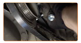
Screw in the lower fastener of the alternator. Use a drive socket #13. Use a drive socket #16. Use a ratchet wrench.
