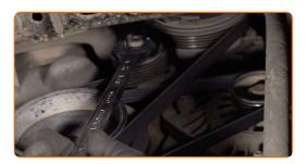
Screw in the fastener of the AC compressor belt tensioner pulley. Use a combination spanner #21. Use HEX No.H7.
