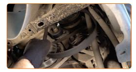
Loosen the lower fastener of the alternator. Use a drive socket #13. Use a drive socket #16. Use a ratchet wrench.
