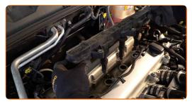
Clean dirt, dust and debris from inside the spark plug wells. Unscrew the spark plugs. Use the spark plug socket #16. Use a ratchet wrench.
