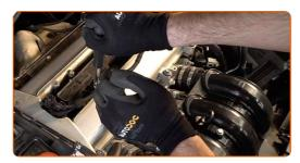
7 Take out the ignition coil from the spark plug well.
