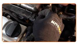
Install the engine cover and secure it. Use a drive socket #8. Use a ratchet wrench.
