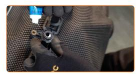
Install the ignition coil to the spark plug well. Make sure you hear a click indicating that it is locked in place.
