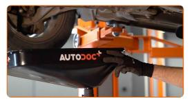
6 Clean the area of the oil pan drainage hole. Use all-purpose cleaning spray.
