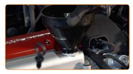
Pour oil into the engine through the filler. Required amount of oil: 5.4 L.
