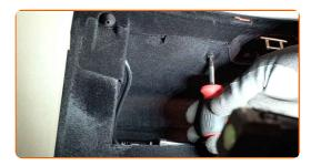
Unscrew the fasteners of the cabin filter housing cover. Use a drive socket #5.5.
