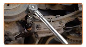
18 Remove the mounting from under the rear axle beam.
