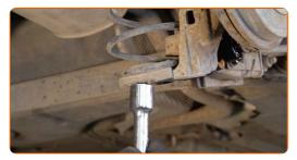
Unscrew the lower fastener of the shock absorber. Use a drive socket #21.
