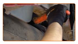
Pull down the rear suspension beam. Use a crowbar.
