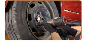
Lower the car and working in a cross order, tighten the wheel bolts. Use a torque wrench. Tighten it to 90 nm torque.
