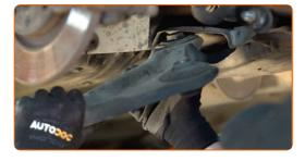
Clean the mounting seats and the thread of the suspension arm. Use a wire brush.
