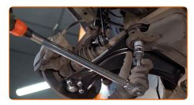
Tighten the rear fastener of the control arm. Use 12-point socket No.22. Use a torque wrench. Tighten it to 126 Nm torque.
