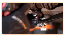
Screw the rear arm fastener. Use 12-point socket No.22.
