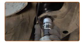
Screw the front arm fastener. Use 12-point socket No.22.
