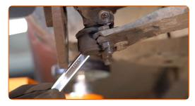
Remove the fastening bolt.
