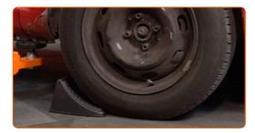
6 Loosen the wheel mounting bolts. Use wheel impact socket #17.
