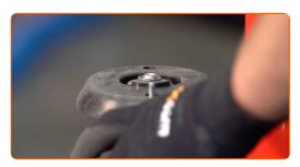
Tighten the shock strut piston rod nut. Use HEX No.H7. Use a drive socket #19. Use a torque wrench. Tighten it to 60 Nm torque.
