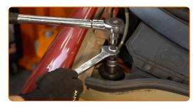
71 Treat the shock strut fasteners. Use copper grease.
