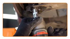
Disconnect the spherical joint from the arm.
