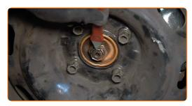
Tighten the upper fastener of the shock absorber strut mount. Use a drive socket #22. Use HEX No.H7. Use a torque wrench. Tighten it to 60 nm torque.
