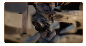
Unscrew the fastener connecting the drive shaft to the wheel hub. Use a drive socket #30.
