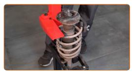
Remove the strut piston rod nut. Use a drive socket #19. Use HEX No.H7. Use a ratchet wrench.
