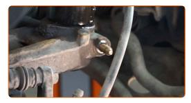
Screw in the fastener that connects the shock strut to the steering knuckle. Use a drive socket #16.
