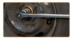
Tighten the wheel bolts using a criss-cross pattern. Use a torque wrench. Tighten it to 90 Nm torque.
