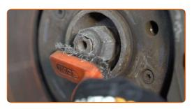
Unstake the fastener of the driveshaft. Use a flat metal-working chisel. Use a hammer.
