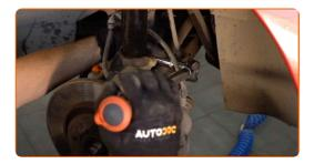
Tighten the fastener connecting the stabilizer link to the shock strut. Use a drive socket #17. Use a torque wrench. Tighten it to 35 Nm torque.
