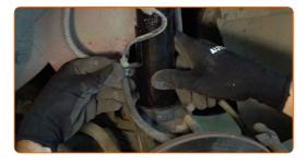
Tighten the lower fasteners connecting the shock strut to the steering knuckle. Use a drive socket #16. Use a torque wrench. Tighten it to 59 Nm torque.
