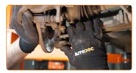
Screw the fasteners of the ball joint. Use a drive socket #16.
