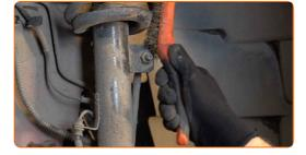
Disconnect the wiring and the brake hose from the bracket on the shock strut. Use a crowbar.
