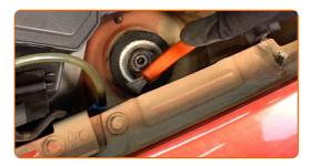
Loosen the upper fastener of the shock strut mount. Use HEX No.H7. Use a combination spanner #22. Use a ratchet wrench.
