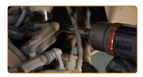
Remove the fastening bolt.
