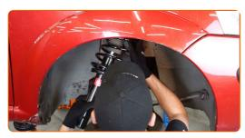
Screw the top fastening of the shock strut mount. Do not tighten it.
