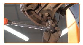
Screw the nut of the drive shaft. Use a drive socket #30.
