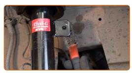
12 Install a new rod, tighten the fasteners.
