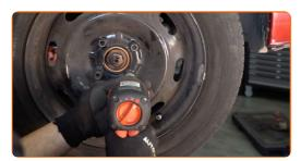
Lower the car and working in a cross order, tighten the wheel bolts. Use wheel impact socket #17. Use a torque wrench. Tighten it to 90 nm torque.
