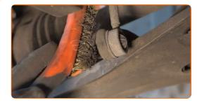
Unscrew the fastener connecting the stabilizer link to the stabilizer bar. Use a combination spanner #17. Use Torx T30. Use a ratchet wrench.
