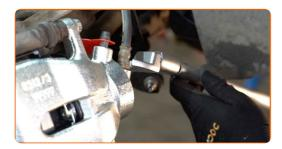
Undo the brake bleeder screw. Use a combination spanner #8.
