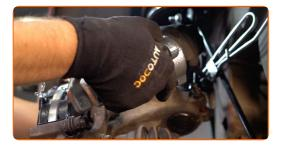
Tighten the brake hose fastener. Use a combination spanner #14.
