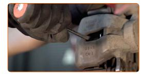
14 Remove the brake caliper.
