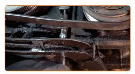
Tighten the tensioner lever of the V-ribbed belt. Use a drive socket #13. Use a torque wrench. Tighten it to 19 Nm torque.
