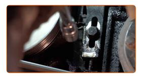
Pull aside the V-ribbed belt tensioner pulley. Use a drive socket #10. Use a ratchet wrench.
