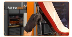
Snap on the circlip connecting the gas strut to the car body.
