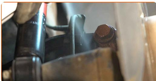
**37** Install the coil spring together with the rubber mounts into the mounting seats.
