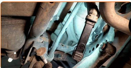
**22** Remove the fastening bolt. Use a drive socket #21.
