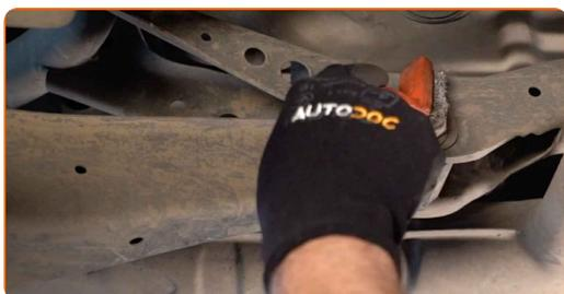
**7** Make a mark on the camber adjustment bolt.
