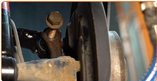
**29** Screw in the fasteners connecting the control arm to the rear knuckle. Use a drive socket #21. Use a combination spanner #21.
