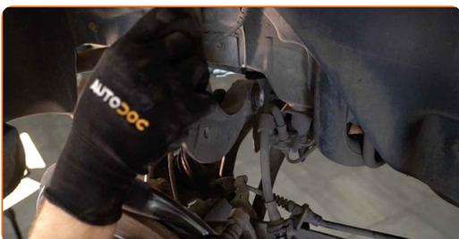
**24** Clean the mounting seats and the thread of the suspension arm. Use a wire brush. Use WD-40 spray.
