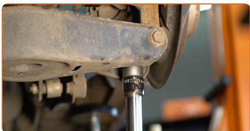
**31** Tighten the fastener connecting the control arm to the rear subframe. Use a combination spanner #18. Use a drive socket #18. Use a torque wrench. Tighten it to 95 Nm torque.
