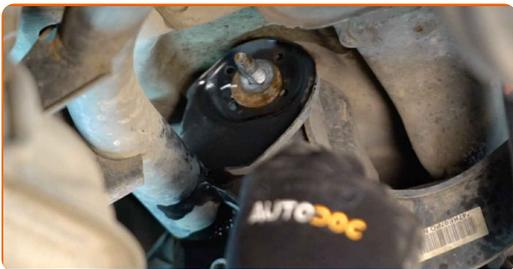
**21** Remove the fastening bolt. Use a crowbar. Use a hammer.
