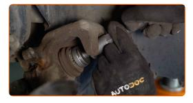
Install the brake caliper and fix it. Use a drive socket #13. Use a combination spanner #13. Use a torque wrench. Tighten it to 35 Nm torque.
