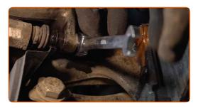
Remove the brake caliper. Use a crowbar.
