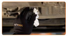
16 Screw in the new drainage plug and tighten it. Use a drive socket #19. Use a torque wrench. Tighten it to 30 Nm torque.
