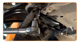
Tighten the rear fastener of the control arm. Use a drive socket #18. Use a torque wrench. Tighten it to 120 Nm torque.
