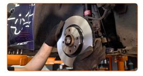
Tighten the brake disc fastening. Use Torx T30. Use a torque wrench. Tighten it to 9 Nm torque.
