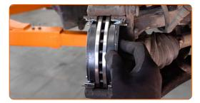
Install the brake caliper and fix it. Use a combination spanner #13. Use a drive socket #13. Use a torque wrench. Tighten it to 30 Nm torque.
