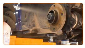
Install the brake disc.
