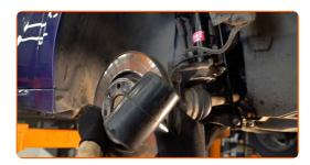
Clean the hub. Use a wire brush. Treat the contacting surface. Use copper grease.
