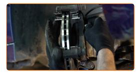
Tighten the brake caliper bracket. Use Torx T55. Use a torque wrench. Tighten it to 105 Nm torque.
