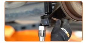
Tighten the lower fastener of the shock absorber. Use a drive socket #16. Use a combination spanner #16. Use a torque wrench. Tighten it to 40 Nm torque.+90°
