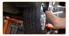
6 Unscrew and remove the wheel arch cover fasteners. Use Torx T25.
