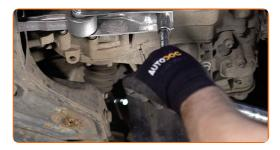
Use a drive socket #16. Use a torque wrench. Tighten it to 40 Nm torque.+90°
