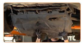
Screw in the fasteners of the lower sound insulation. Use a drive socket #12. Use a Phillips screwdriver.
