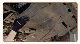
6 Clean the engine mount fasteners. Use a wire brush. Use WD-40 spray.
