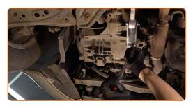
13.1 Tighten the engine mount fastening bolts.
