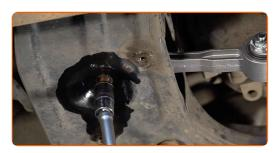
Screw in the engine mount fastener that connects it to the gearbox housing. Use a drive socket #16. Use a ratchet wrench.
