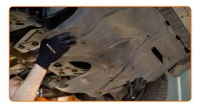
Put a waste oil container with at least 4 l capacity under the drainage hole.
