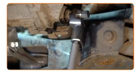
Insert the funnel. Pour the oil into the gearbox through the filler hole. Required amount of oil: 1.5 L.
