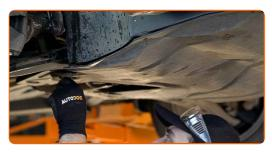
Remove the lower sound insulation.
