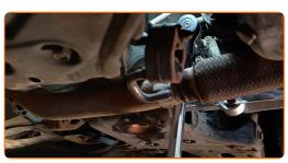
Clean the area around the gearbox housing filler hole. Use all-purpose cleaning spray.
