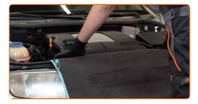
Remove the engine cover. The air filter housing is integrated into the engine cover.
