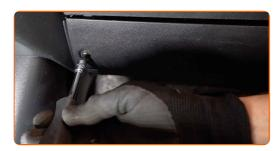
$\Lambda$  Pry up, carefully release from the fasteners and remove the side trim panel on the passenger side.
