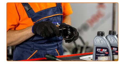
Remove the old seal of the oil filter cap Use a flat screwdriver.
