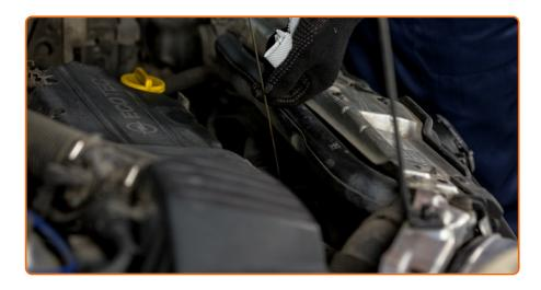
Check the oil level using the dipstick. Top up oil if necessary.
