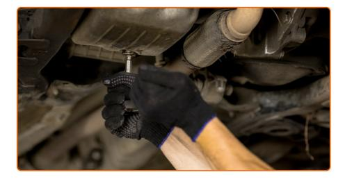
Screw in the new drainage plug and tighten it. Use Torx T55. Use a torque wrench. Tighten it to 30 Nm torque.
