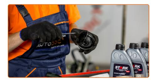
Install a new seal of the oil filter cap Use a flat screwdriver.
