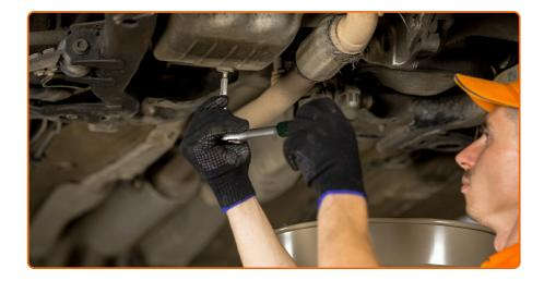
Unscrew the drain plug. Use Torx T55. Use a ratchet wrench.
