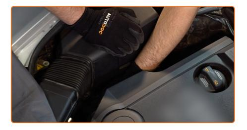
Lock the retaining clips of the air filter housing cover.
