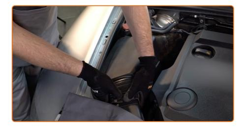
Reinstall the air filter cover. Fasten it.
