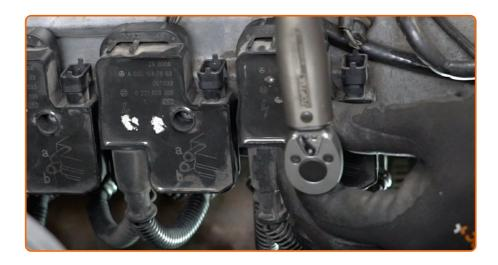
Tighten the ignition coil fasteners. Use Torx T30. Use a torque wrench. Tighten it to 18 nm torque.
