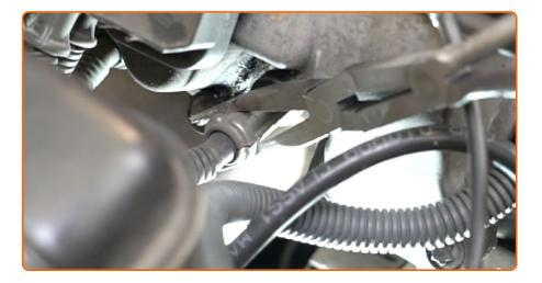
Remove the spark plug wire connectors from the spark plug wells. Use long round nose pliers.
