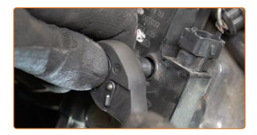
Unscrew the fasteners of the ignition coils. Use Torx T30. Use a ratchet wrench.
