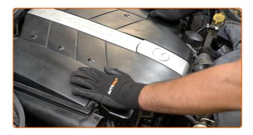
Install the engine cover and secure it.
