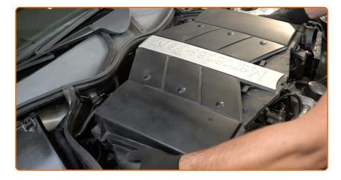
Remove the air filter housing.
