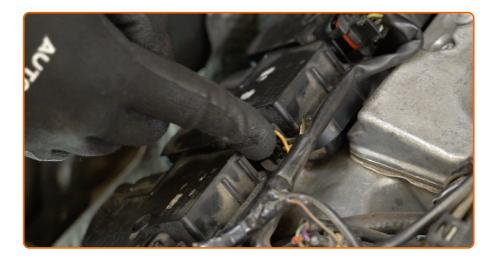
Plug in the connectors of the ignition coils. Make sure you hear a click indicating that it is locked in place.
