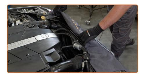
Remove the fender protection cover.
