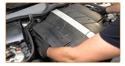
Install the air filter housing.
