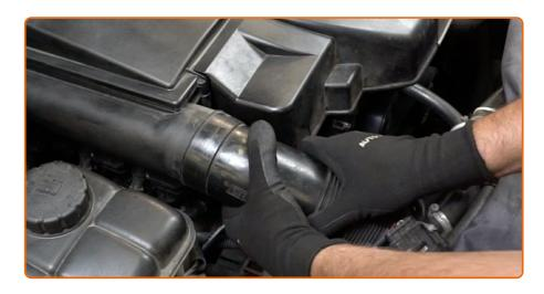
Reinstall the air intake hoses.
