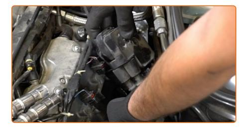
Install the ignition coils to the spark plug wells.
