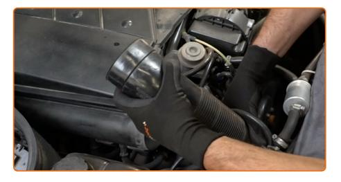
Remove the air intake hoses.
