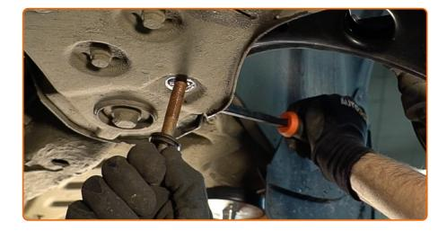
Install the control arm fasteners.
