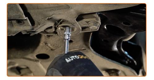
Install and tighten the wheel arch cover fasteners. Use a Phillips screwdriver. Use a drive socket #10. Use a ratchet wrench.
