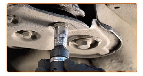
Unscrew the rear arm fastener. Use a drive socket #19. Use a tap wrench.
