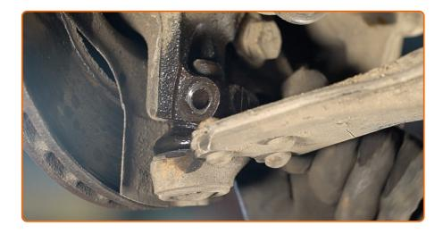
Remove the fastening bolt.
