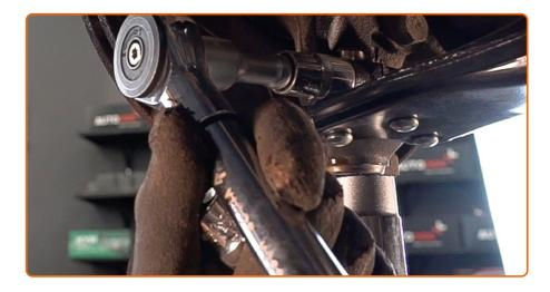
Tighten the ball joint fastener. Use a drive socket #17. Use a combination spanner #17. Use a torque wrench. Tighten it to 65 nm torque.
