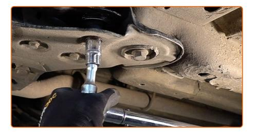
Tighten the rear fastener connecting the arm to the body subframe. Use a drive socket #19. Use a torque wrench. Tighten it to 75 nm torque.
