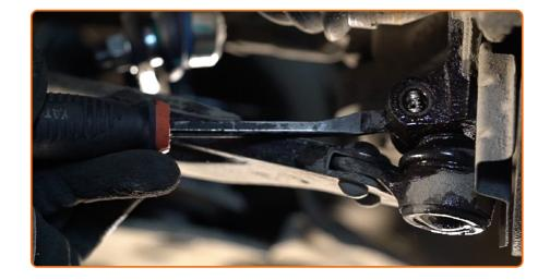
Release the fastener connecting the ball joint to the steering knuckle. Use a crowbar. Use a hammer.
