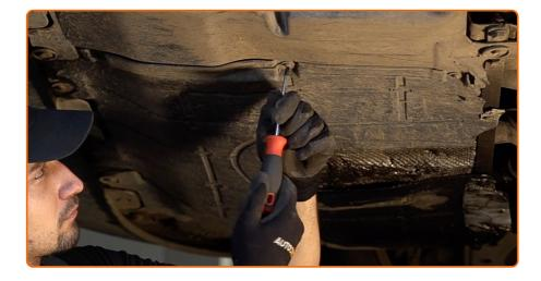
Unscrew and remove the wheel arch cover fasteners. Use a Phillips screwdriver. Use a drive socket #10. Use a ratchet wrench.
