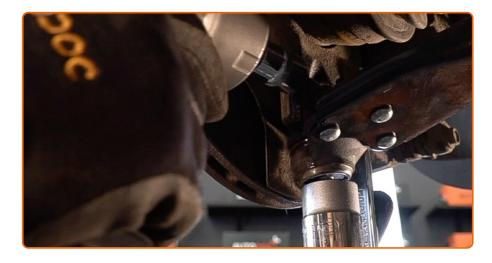
Screw the fastener connecting the ball joint to the steering knuckle. Use a drive socket #17. Use a combination spanner #17.
