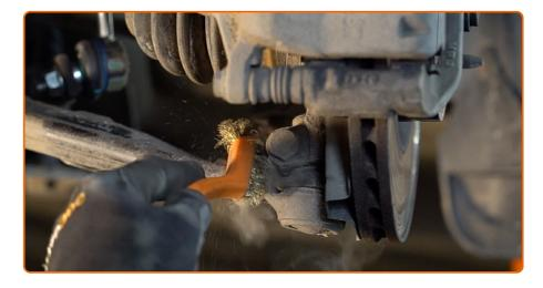
Clean the fastener connecting the ball joint to the steering knuckle. Clean all joints of the arm. Use a wire brush. Use WD-40 spray.
