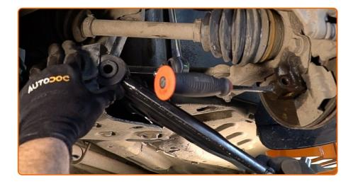
Install a new arm. Use a pin punch.
