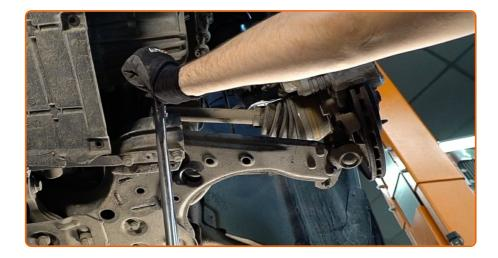
Unscrew the front arm fastener. Use a drive socket #21. Use a tap wrench.
