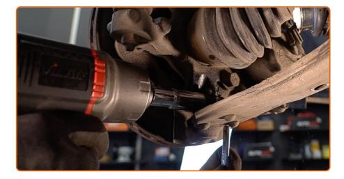
Unscrew the ball joint fastening to the steering knuckle. Use a combination spanner #17. Use a drive socket #17. Use a ratchet wrench.
