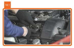
Connect the plugs to the ignition coil.
