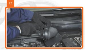
Remove the air supply pipe.
