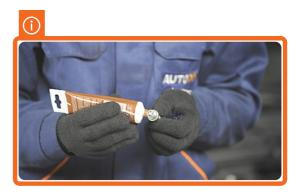
Apply a thin layer of special grease on the thread surface of new spark plugs.
