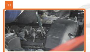
Unscrew the ignition coil fastening screws.
