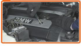
Remove the bolts and take off the plastic engine cover
