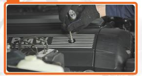
Screw the fastening bolts of the plastic engine cover
