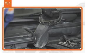
Install the air supply pipe and fasten it.
