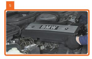
Remove the cylinder head cover.
