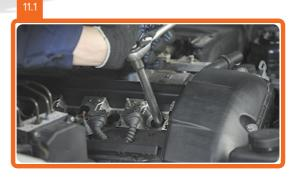
Remove the spark plugs with a spark plug wrench and place them on a work surface in the order of installing in the engine.
