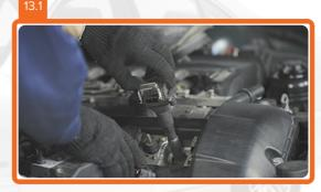
Put the ignition coils onto the spark plugs and secure.
