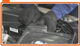
Connect the pipes and hoses to the air filter housing.
