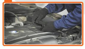
Disconnect the pipes and hoses from the air filter housing.
