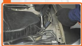
Screw the filter housing fastening bolts.
