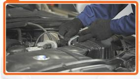
Disconnect the wiring from the mass air flow sensor.
