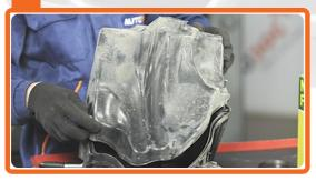
Reinstall the air filter cover. Fasten it.
