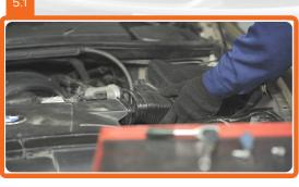
Remove the air filter housing.
