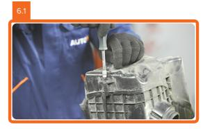
Loosen and remove the air filter cover.
