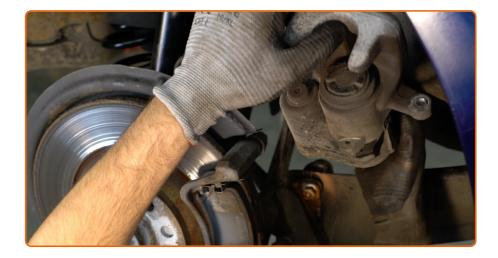
Remove the brake caliper.
