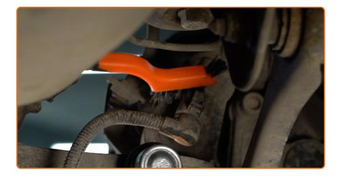
Clean the parking brake connector. Use a wire brush. Use all-purpose cleaning spray.
