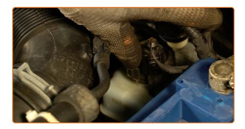
Tighten the brake fluid reservoir cap.
