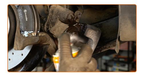
Treat the brake caliper piston. Use a brake cleaner.
