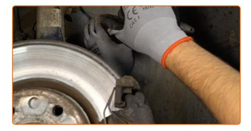
Unscrew the wheel arch cover fasteners. Use Torx T25. Use a ratchet wrench.
