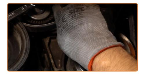
Pull aside the V-ribbed belt tensioner pulley. Use a combination spanner #16.
