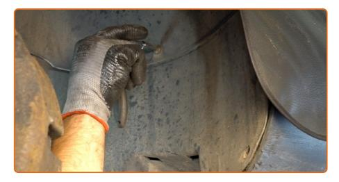
Install and tighten the wheel arch cover fasteners. Use Torx T25. Use a ratchet wrench.
