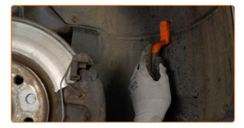
Clean the fasteners of the locker. Use a wire brush.
