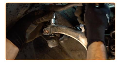
Screw on the fastening nut that connects the tie rod end to the steering knuckle. Use a drive socket #13. Use a ratchet wrench.
