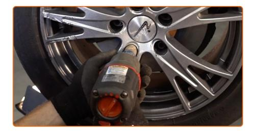
Screw in the wheel bolts. Use wheel impact socket #17.
