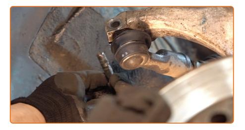
Remove the fastening bolt. Use a flat metal-working chisel. Use a hammer.
