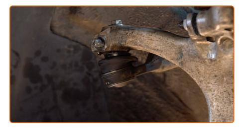
Unscrew the end fastening nut to the steering knuckle. Use a drive socket #13. Use a ratchet wrench.
