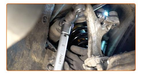
Tighten the tie rod end locknut. Use a combination spanner #18. Use a combination spanner #22. Use a torque wrench. Tighten it to 55 nm torque.
