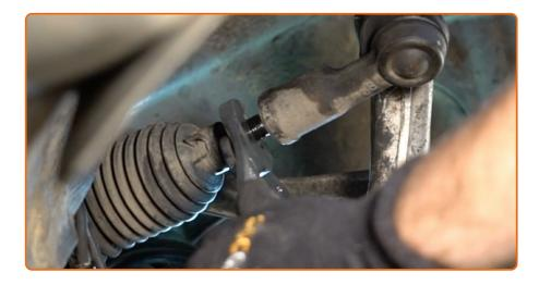
Loosen the lock nut securing the tie rod end to the tie rod. Use a combination spanner #18. Use a combination spanner #22.
