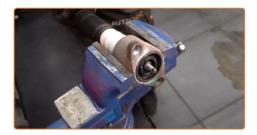
Install the mount, boot and bump stop onto a new shock absorber.
