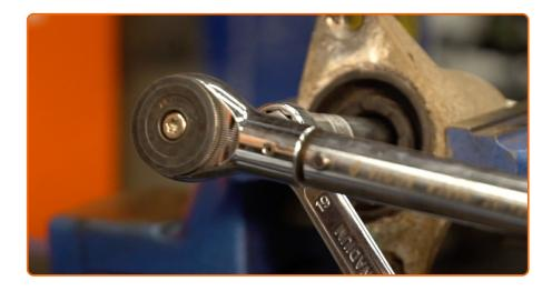
Screw the shock strut piston rod upper fastening. Use a shock absorber socket DDN°6. Use a drive socket #16. Use a torque wrench. Tighten it to 50 Nm torque.
