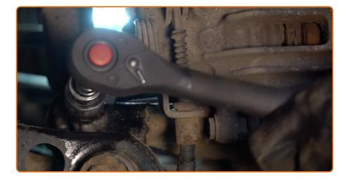
Unscrew the lower fastener of the shock absorber. Use a combination spanner #21. Use a drive socket #21. Use a ratchet wrench.
