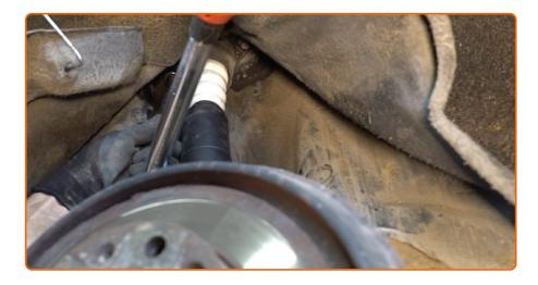
Tighten the top shock absorber fastening. Use a drive socket #13. Use a torque wrench. Tighten it to 48 Nm torque.
