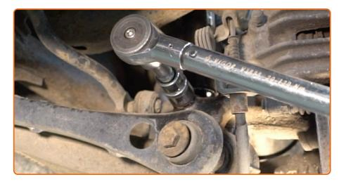
Tighten the lower fastener of the shock absorber. Use a combination spanner #21. Use a drive socket #21. Use a torque wrench. Tighten it to 80 Nm torque.
