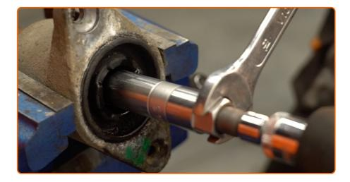
Remove the shock absorber piston rod fastening. Use a shock absorber socket DDN°6. Use a drive socket #16. Use a ratchet wrench.
