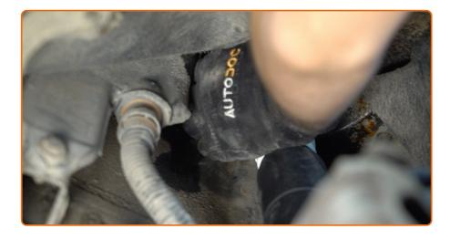
Screw the upper fastener of the shock absorber. Use a drive socket #13.
