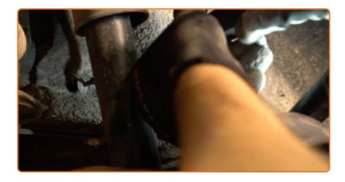
Unscrew and remove the wheel arch cover fasteners. Use Torx T25.
