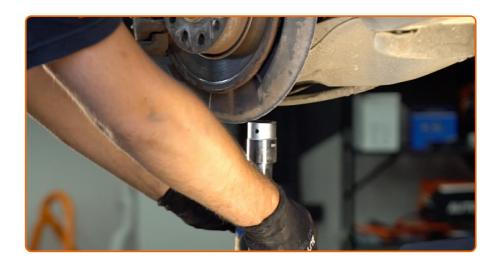
Remove the support from under the arm.
