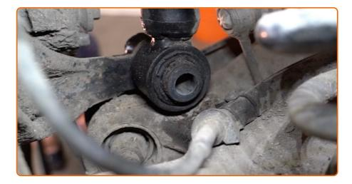
Remove the fastening bolt.
