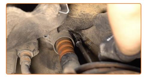
Unscrew the upper fastener of the shock absorber. Use a drive socket #13. Use a ratchet wrench.
