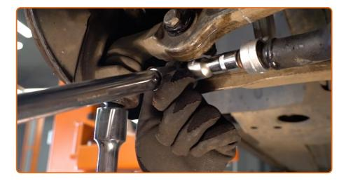
Tighten the fastener connecting the stabilizer link to the stabilizer bar. Use a combination spanner #16. Use a drive socket #16. Use a torque wrench. Tighten it to 65 Nm torque.
