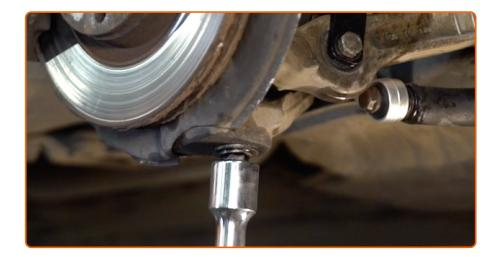
Remove the support from under the arm.
