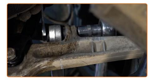
install the rod fastening to the stabilizer and tighten it. Use a combination spanner #16. Use a drive socket #16. Use a torque wrench. Tighten it to 65 Nm torque.
