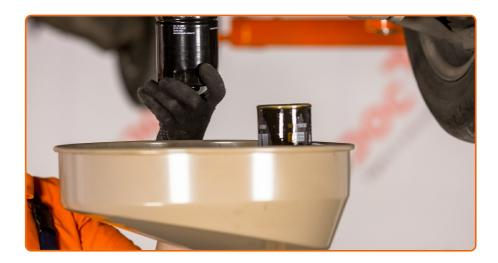
Screw the new filter into its place. Use the 67-14F socket. Use a torque wrench. Tighten it to 25 Nm torque.
