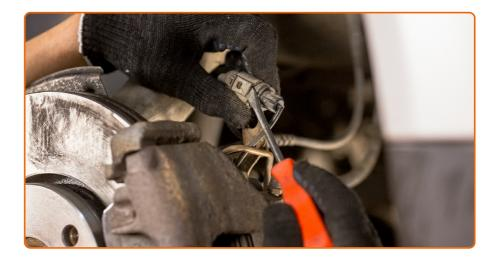
Connect the brake pad wear sensor plug.
