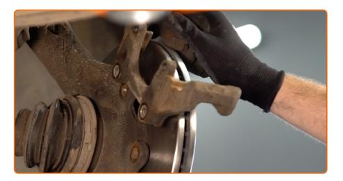
Remove the caliper bracket
