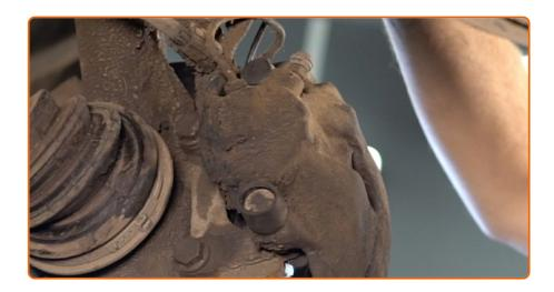
Disconnect the brake pad wear sensor plug. Use a flat screwdriver.
