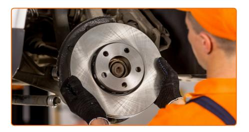
Install the brake disc.
