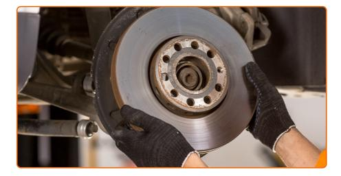
Remove the brake disc.
