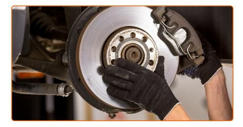
Remove the brake caliper.
