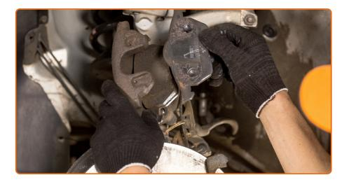
Remove the brake pads.
