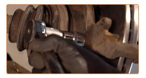
Install the brake caliper bracket
