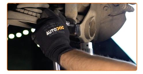
Unscrew the lower fastener of the shock absorber. Use a combination spanner #16. Use a drive socket #16. Use a ratchet wrench.
