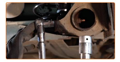
Tighten the lower fastener of the shock absorber. Use a combination spanner #16. Use a drive socket #16. Use a torque wrench. Tighten it to 80 Nm torque.
