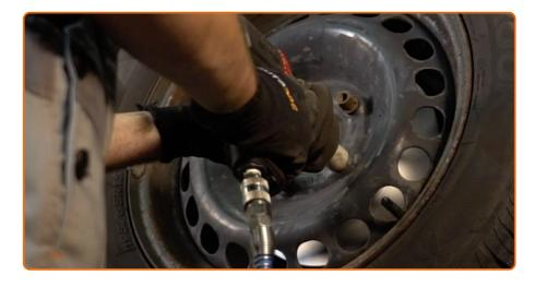
Screw in the wheel bolts. Use wheel impact socket #17.
