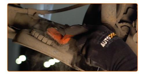
Clean the coil spring mounting seats. Use a wire brush. Use WD-40 spray.
