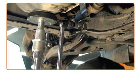
Unscrew the front arm fastener. Use a drive socket #22. Use a tap wrench.
