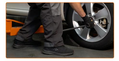
Loosen the wheel mounting bolts. Use wheel impact socket #21.
