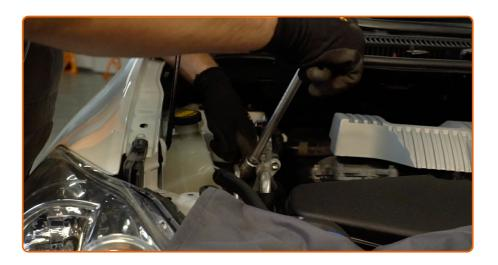
Unscrew the upper fastener of the engine mount. Use a drive socket #17. Use a ratchet wrench.
