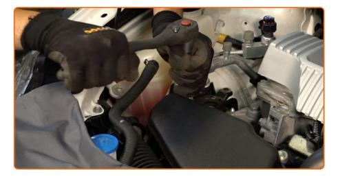
Tighten the upper fastener of the engine mount. Use a drive socket #17. Use a torque wrench. Tighten it to 75 nm torque.
