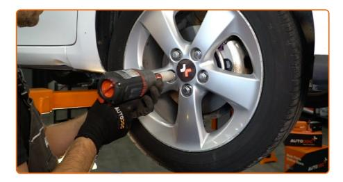
Screw in the wheel bolts. Use wheel impact socket #21.
