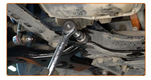
Tighten the front fastener connecting the control arm to the subframe. Use a drive socket #22. Use a torque wrench. Tighten it to 80 Nm torque.
