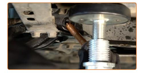
Install the front fastener of the arm.
