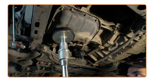
Support the engine in the oil pan area.
