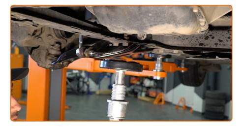
Remove the hydraulic transmission jack.
