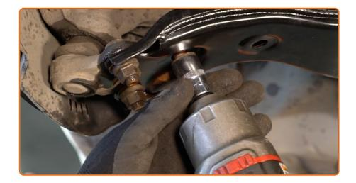
Screw the fasteners of the ball joint. Use a drive socket #17. Use a ratchet wrench.
