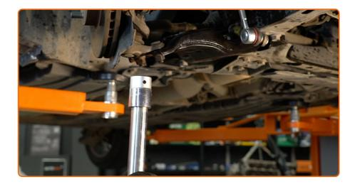
Remove the support from under the arm.
