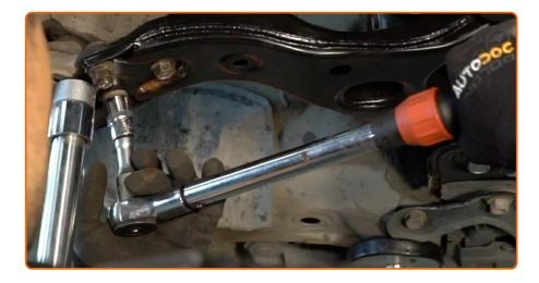
Tighten the ball joint fastener. Use a drive socket #17. Use a torque wrench. Tighten it to 50 nm torque.
