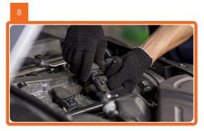
Connect the plugs to the ignition coil.
