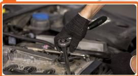
Remove the spark plugs with a spark plug wrench and place them on a work surface in the order of installing in the engine.
