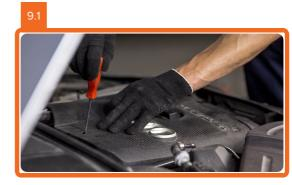
Install the engine cover and secure it.
