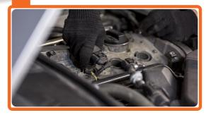
Install the ignition coil straight down.
