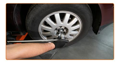
Unscrew the hub lock nut. Use 1-3/16" drive 12-point socket.
