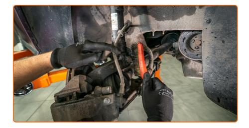
Clean the fasteners connecting the shock strut to the steering knuckle. Clean the fasteners connecting the ball joint to the suspension control arm. Use a wire brush. Use WD-40 spray.
