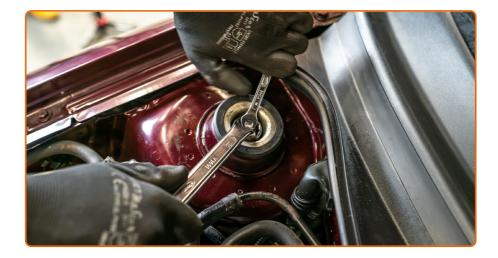
Tighten the upper fastening nut of the shock absorber strut. Do not tighten it.
