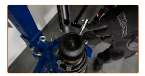
Remove the strut piston rod nut. Use flare nut socket #22. Use HEX No.H6.
