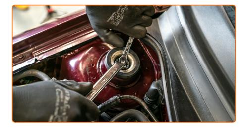
Tighten the shock strut top mount. Use a drive socket #22. Use a torque wrench. Tighten it to 60 Nm torque.
