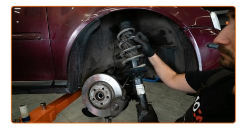
Remove the suspension strut. Set the shock absorber strut on the spring compressor tool.
