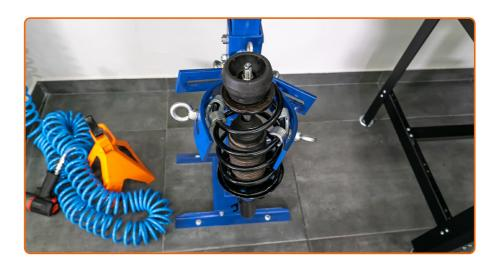
Tighten the shock strut piston rod nut. Use flare nut socket #22. Use HEX No.H6. Use a torque wrench. Tighten it to 60 Nm torque.
