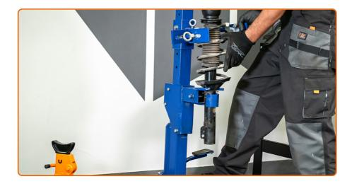
Release the coil spring.
