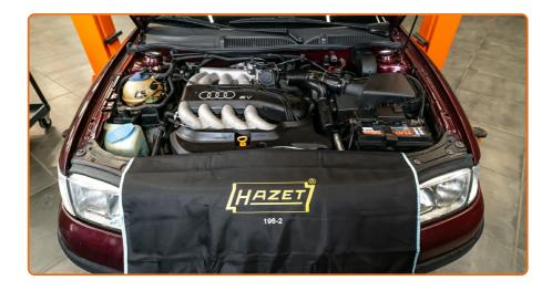
Remove the fender protection cover.
