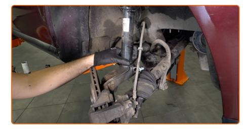
Disconnect the steering knuckle from the shock absorber strut.
