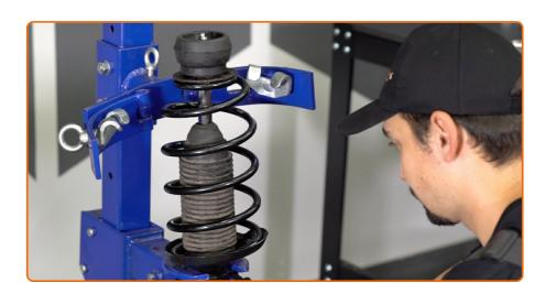
Remove the assembled shock strut.
