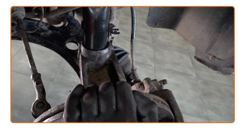
Treat the shock strut mounting seat on the steering knuckle. Use WD-40 spray.
