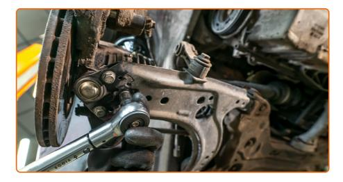
Screw in the fasteners of the ball joint lock plate (3 pieces). Use a drive socket #13. Use a torque wrench. Tighten it to 45 Nm torque.
