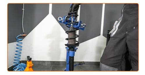
Install the spring on the shock absorber.
