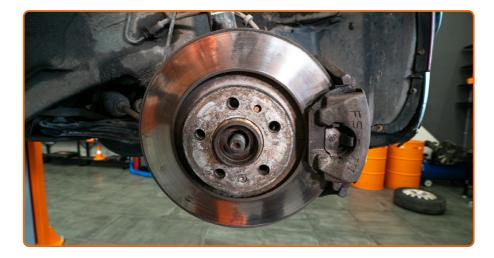
Unscrew the fastener connecting the drive shaft to the wheel hub. Use 1-3/16" drive 12-point socket.
