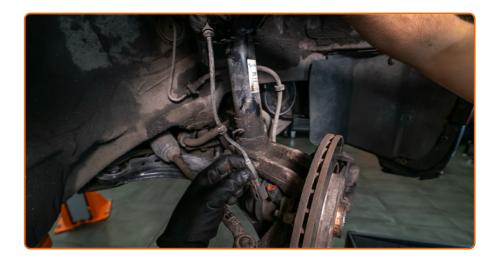
Fasten the brake hose on the strut. Connect the fastener of the ABS sensor cable to the shock absorber strut.
