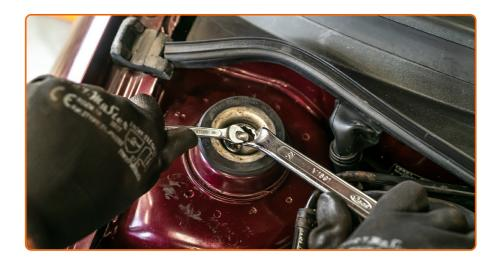
Unscrew the upper fastening of the shock absorber strut. Use a combination spanner #21. Use HEX No.H6.
