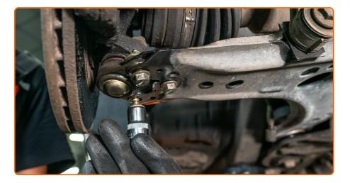
Unscrew the fastener connecting the ball joint to the suspension control arm. Use a drive socket #13.
