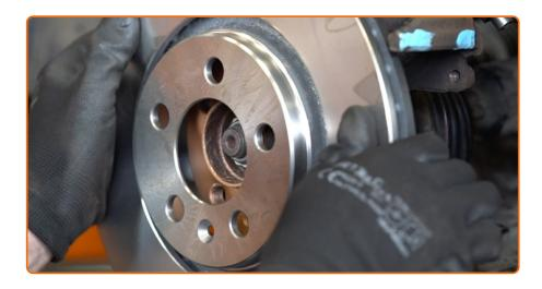
Install the new brake disc on the hub and tighten the screws.
