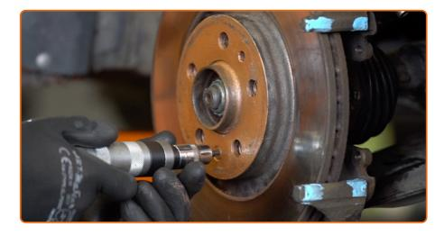
Unscrew the brake disc mounting bolts and remove it. Use Torx T30.
