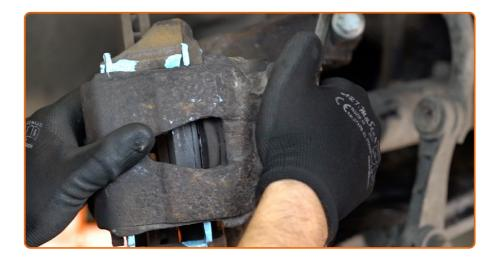
Remove the brake caliper.
