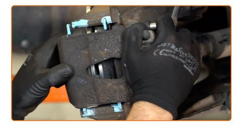
Install the brake caliper and fix it. Use HEX No.H7. Use a torque wrench. Tighten it to 35 Nm torque.
