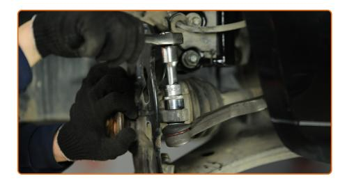
Tighten the fastening nut connecting the tie rod end to the steering knuckle. Use a drive socket #22. Use a torque wrench. Tighten it to 70 nm torque.
