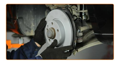
Install the brake disc.
