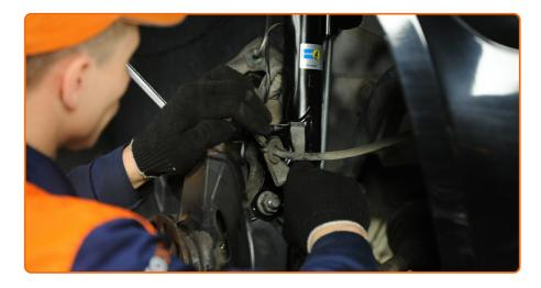
Install the bracket onto the shock absorber strut.
