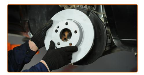
Remove the brake disc.
