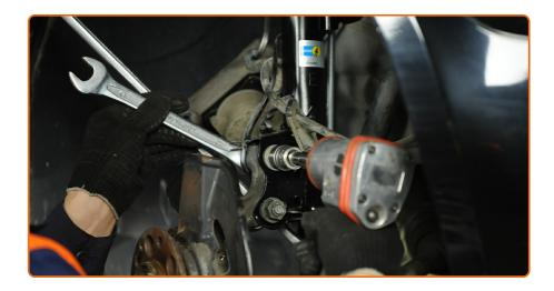
Tighten the lower fasteners connecting the shock strut to the steering knuckle. Use a combination spanner #21. Use a drive socket #21. Use a torque wrench. Tighten it to 95 Nm torque.
