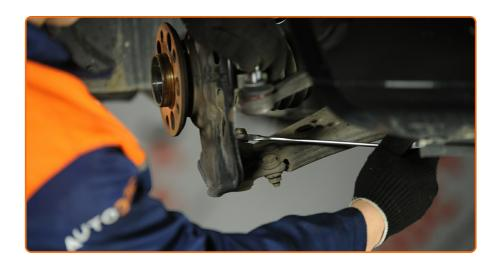
Unscrew the ball joint fastening to the steering knuckle. Use a combination spanner #21.
