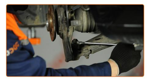
Tighten the ball joint fastener. Use a combination spanner #21. Use a torque wrench. Tighten it to 60 nm torque.
