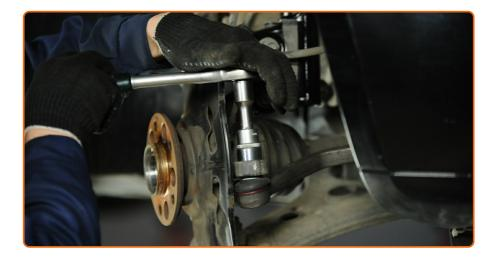
Unscrew the end fastening nut to the steering knuckle. Use a drive socket #22. Use a ratchet wrench.
