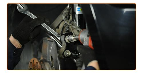
Unscrew the lower fastener connecting the shock strut to the steering knuckle. Use a combination spanner #21. Use a drive socket #21. Use a ratchet wrench.
