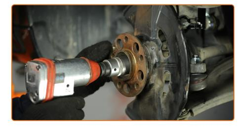
Tighten the hub. Use a drive socket #30. Use a torque wrench. Tighten it to 170 nm torque.
