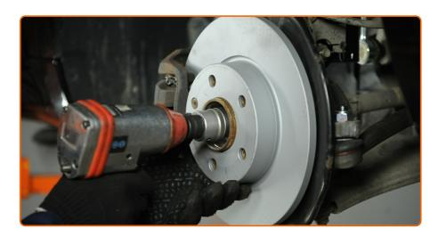
Unscrew the wheel hub axle nut. Use a drive socket #30.
