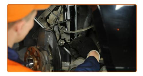
Remove the bracket from the shock absorber strut. Use a flat screwdriver.
