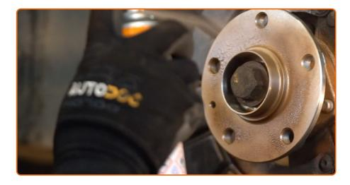
Treat the contacting surface. Use copper grease.
