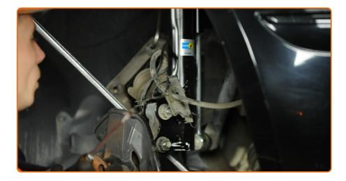
Disconnect the lower arm from the steering knuckle. Use a crowbar. Use a hammer.
