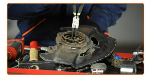
Remove the retaining ring from the steering knuckle. Use circlip pliers.
