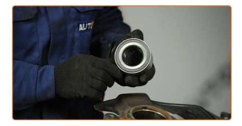
Clean the hub bearing mounting seat. Use a wire brush.
