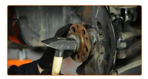
Install the hub bearing protection cap. Use a hammer.
