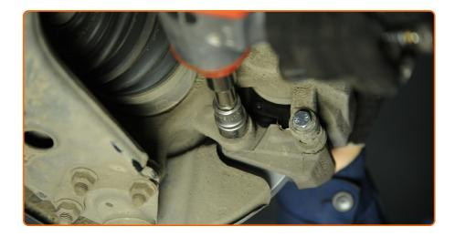
Unscrew the caliper bracket fastening. Use a drive socket #18. Use a ratchet wrench.
