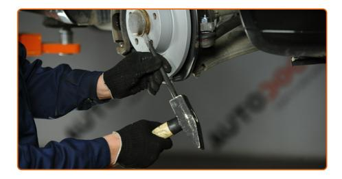
Remove the hub bearing protection cap. Use a flat metal-working chisel. Use a hammer.
