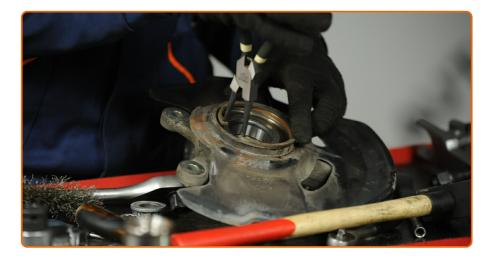
Install the retaining ring in the steering knuckle. Use circlip pliers.
