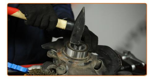
Press the new bearing in the steering knuckle. Use a bush and bearing driver set. Use a hammer.
