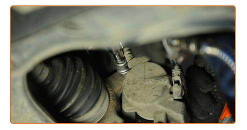
Tighten the brake caliper bracket. Use a drive socket #18. Use a torque wrench. Tighten it to 70 Nm torque.
