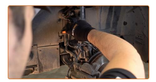
Clean the area where the brake hose is connected to the brake caliper and to the brake circuit pipe.
