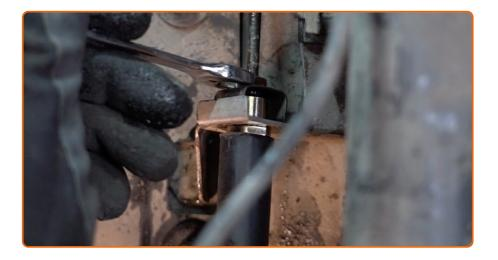
Screw the brake hose onto the brake circuit pipe. Use a combination spanner #11. Use a torque wrench. Tighten it to 22 Nm torque.
