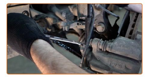
Tighten the fastener connecting the brake pipe to the brake caliper. Use a combination spanner #14. Use a torque wrench. Tighten it to 26 Nm torque.
