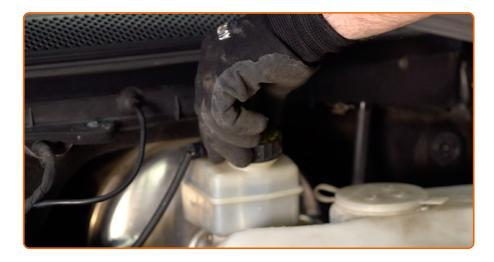
Tighten the brake fluid reservoir cap.
