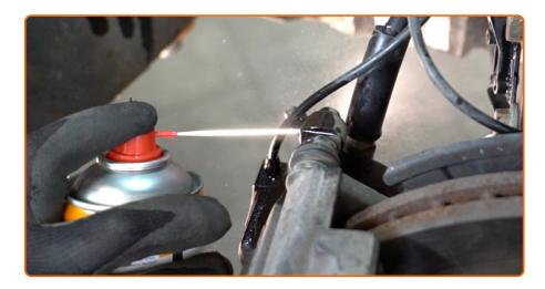
Clean the area where the brake hose is connected to the brake caliper and to the brake circuit pipe. Use a brake cleaner.
