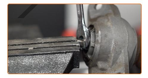
Remove the shock absorber piston rod fastening. Use a combination spanner #14.
