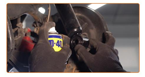
Clean the shock absorber fasteners. Use WD-40 spray.
