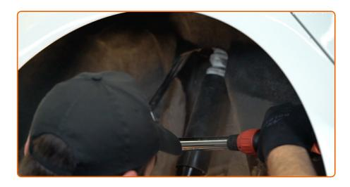
Tighten the shock absorber mount fasteners. Use a drive socket #15. Use a torque wrench. Tighten it to 50 Nm torque.
