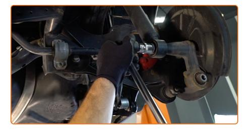
Unscrew the lower fastener of the shock absorber. Use a drive socket #21. Use a tap wrench.
