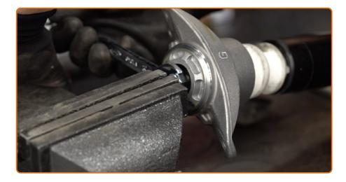
Fix the shock absorber mount. Use a combination spanner #14. Use a drive socket #14. Use a torque wrench. Tighten it to 30 Nm torque.
