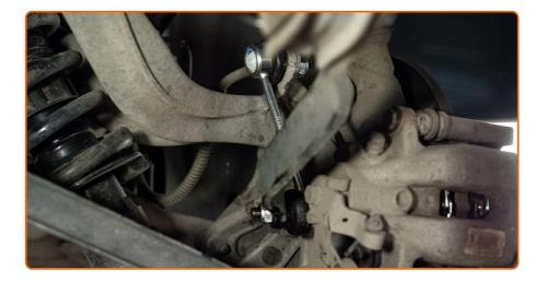
Tighten the fastener connecting the stabilizer link to the stabilizer bar. Use a combination spanner #16. Use Torx T30. Use a torque wrench. Tighten it to 55 Nm torque.
