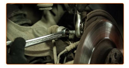
Unscrew the fastener connecting the stabilizer bar with the control arm. Use a combination spanner #16. Use Torx T30. Use a ratchet wrench.
