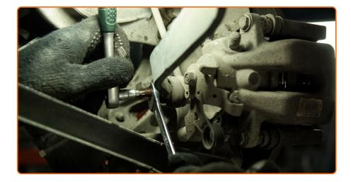
Unscrew the fastener connecting the stabilizer link to the stabilizer bar. Use a combination spanner #16. Use Torx T30. Use a ratchet wrench.
