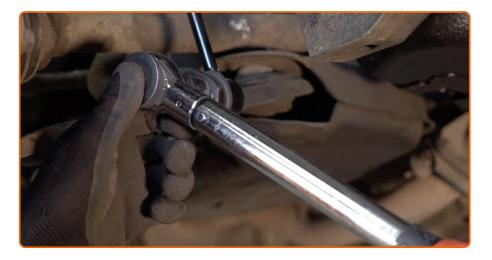
Tighten the fastener connecting the stabilizer bar with the control arm. Use a combination spanner #16. Use Torx T30. Use a torque wrench. Tighten it to 55 Nm torque.
