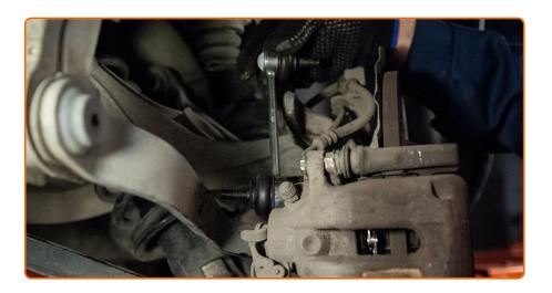
Install a new rod, tighten the fasteners.
