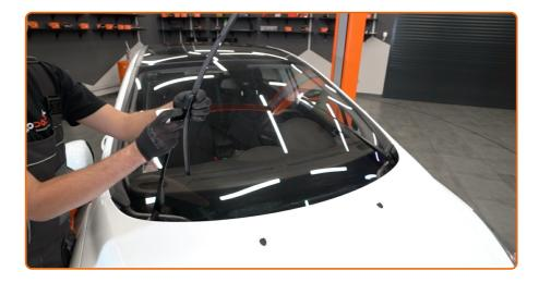
Pull the wiper arm away from the glass surface until it stops.
