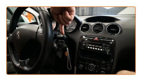
Switch on the ignition. Pull the windscreen wiper stalk to the downward position.
