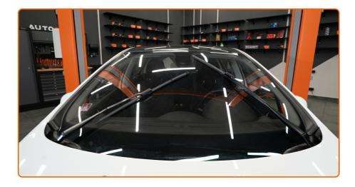
Switch off the ignition. In the service mode, the wipers will be in the upper position.
