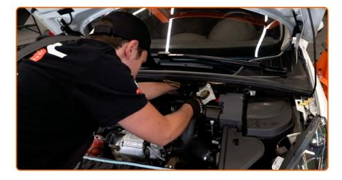
Reinstall the air filter cover. Fasten it.
