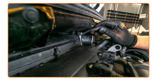
Undo the fastening screws of the air filter cover (3 pieces). Use Torx T25. Use a ratchet wrench.
