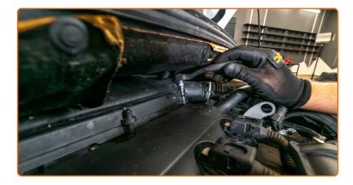
Screw in the fastening screws of the air filter cover (3 pieces). Use Torx T25. Use a ratchet wrench.
