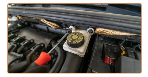
Unscrew the fasteners of the brake fluid reservoir (2 pieces). Use Torx T20.
