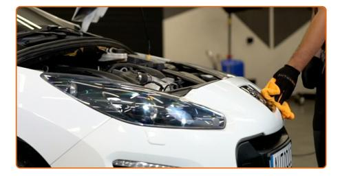
Remove the fender protection cover.
