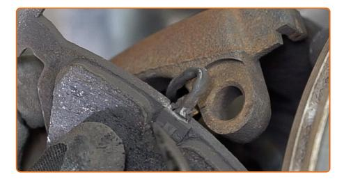
Connect the brake pads wear sensor.
