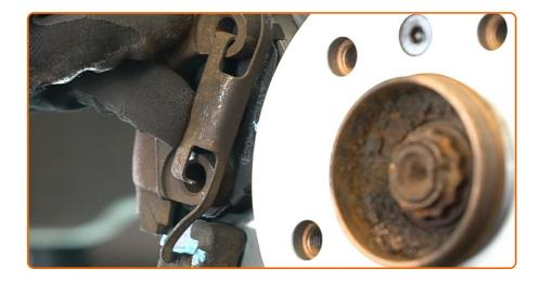
Install the brake caliper retaining spring.
